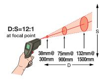
The ST20 XB is ideally used within 2 m of the intended target. At greater distances, the measured area will be larger (approximately the distance divided by twelve).
