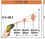
The ST60 XB is ideally used within 5 m of the intended target. At greater distances, the measured area will be larger (approximately the distance divided by 30).
