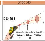
The ST80 XB models are ideally used within 8 m of the intended target. At greater distances, the measured area will be larger (approximately the distance divided by 50).
